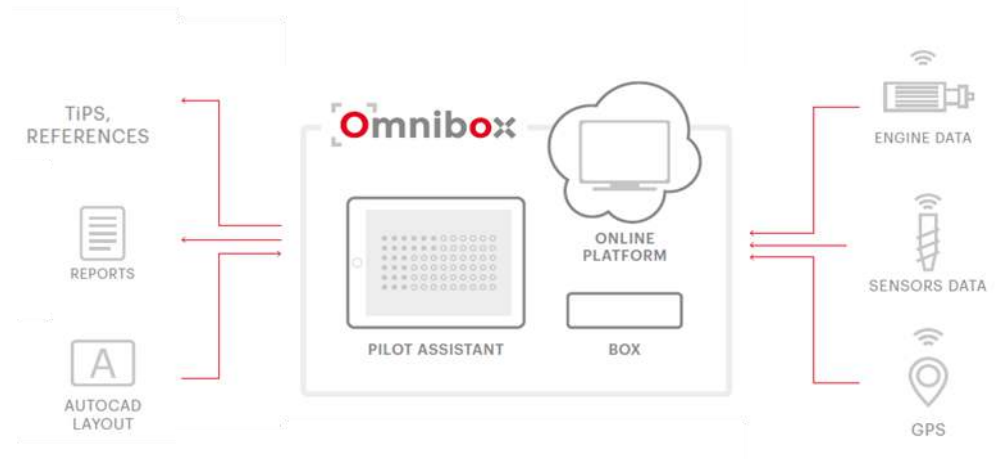
Fig. 1. Sketch explaining the architecture of the OMNIBOX™ solution
